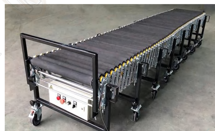
The rollers are driven by V belt
